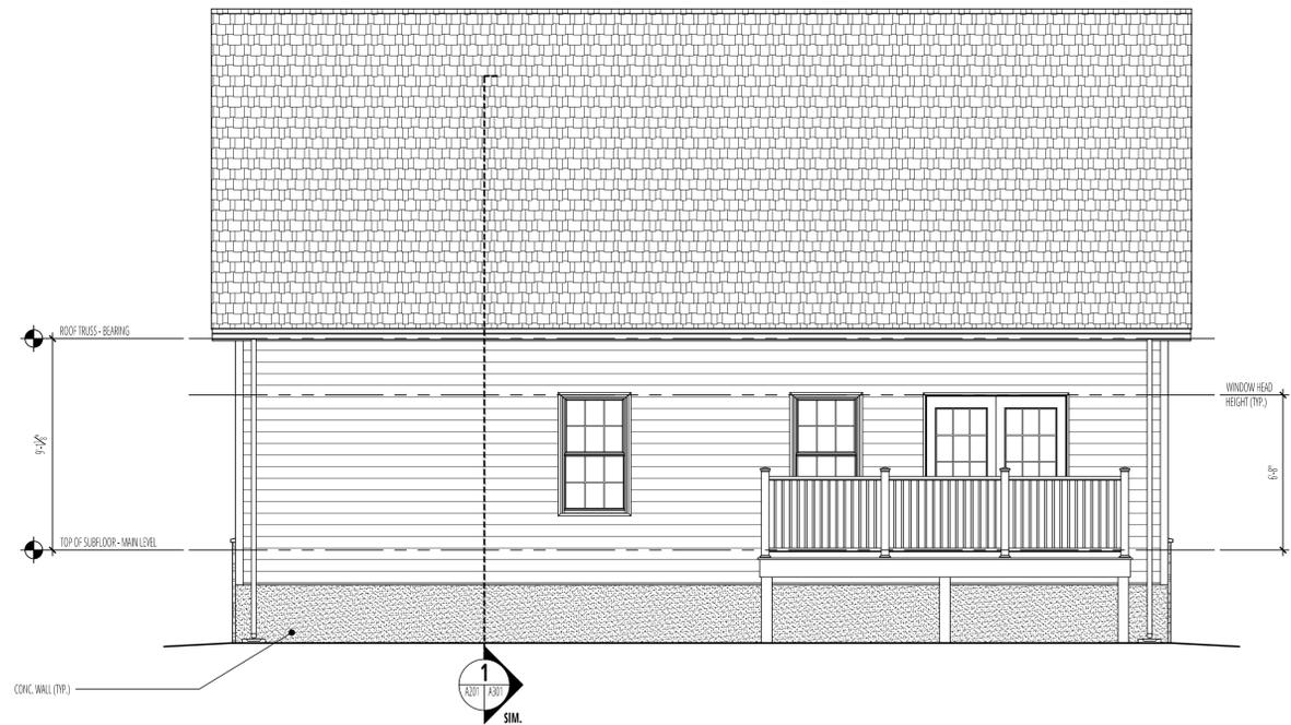
**C** EXTERIOR ELEVATION - REAR - STONE VENEER - OPTION 'A'
